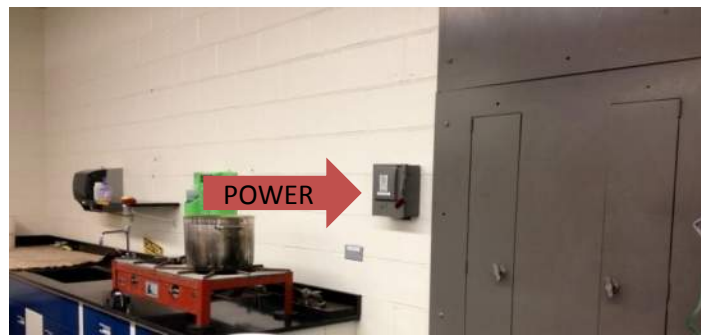
Figure 1. Power Switch Location for Tinius-Olsen Compression Machine
