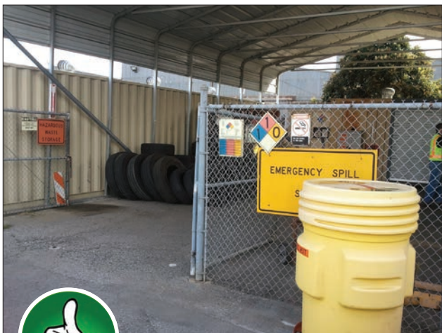
Fig. 3-3. Tires and hazardous waste should always be stored in a covered area whenever possible. Spill response kits should also be kept where they can be accessed if needed.
