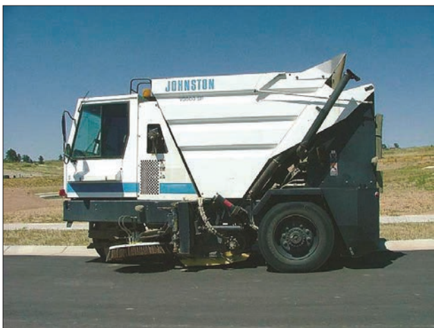
Fig. 2-9. Street sweeping prevents sediment and associated pollutants located on the street surface from discharging with stormwater.
