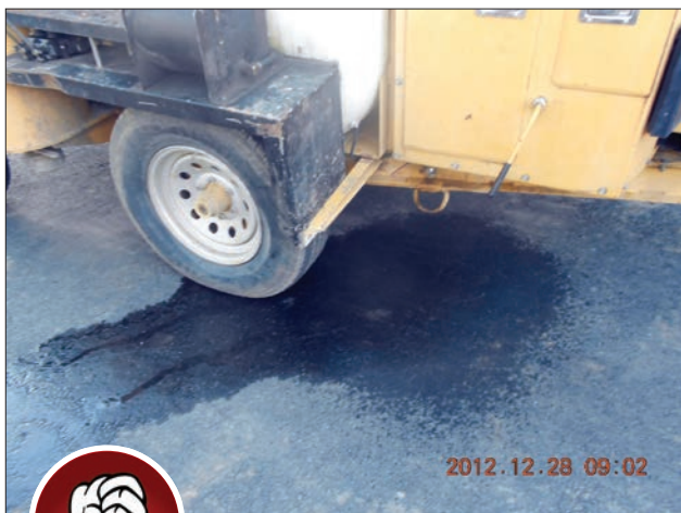
Fig. 3-11. A leak such as this should be cleaned using a damp mop or absorbent cloth. Do not hose down. Source: RBF Consulting
