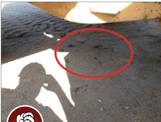
Fig. 3-6. Leaking fuels are a common source of pollutants within vehicle equipment storage areas.
