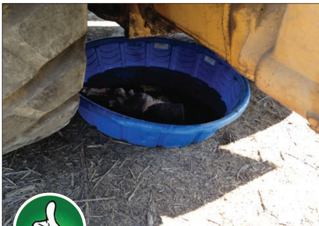
Fig. 3-10. This a good example of using containment to control fuel leaks identified in the field.
