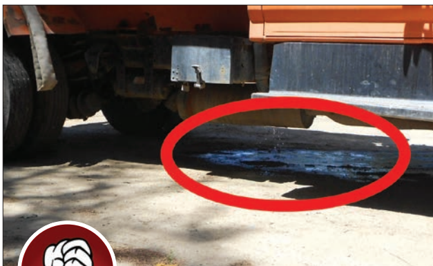
Fig. 2-17. Vehicle leaks are a common non-stormwater discharge. They must be identified and fixed as soon as possible.
