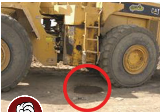
Fig. 2-13. Equipment and vehicles should be inspected routinely for leaks. An ample supply of cleanup materials should be kept at all designated maintenance areas where leaks and spills are likely to occur.
