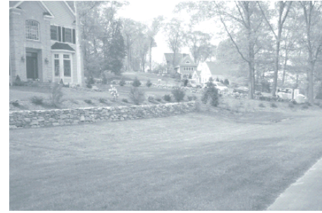
Figure 4.18 – Vegetative filter strip. Source: Connecticut, 2004.
