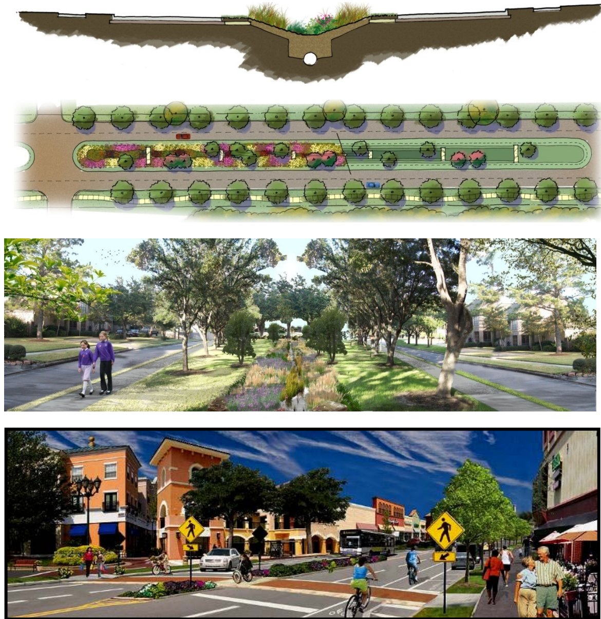
Figure 3.8 – Examples of center median infiltration/filtration systems
