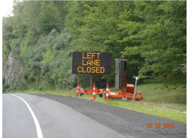
Route 11 SB: A CMS just after Exit 5 stating LEFT LANE CLOSED on its first frame.
