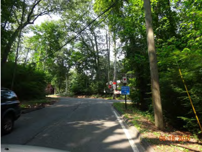
Cobbs Mill Road WB: A blue BUSINESS ACCESS sign notifying that a restaurant near the project site was still open. A DETOUR sign on top of a regulatory Route 57 sign instructing motorists to stay on current route to get to Route 57. This sign may show that the signs on the detour may not be visible enough for motorists to be directed appropriately through the detour.
