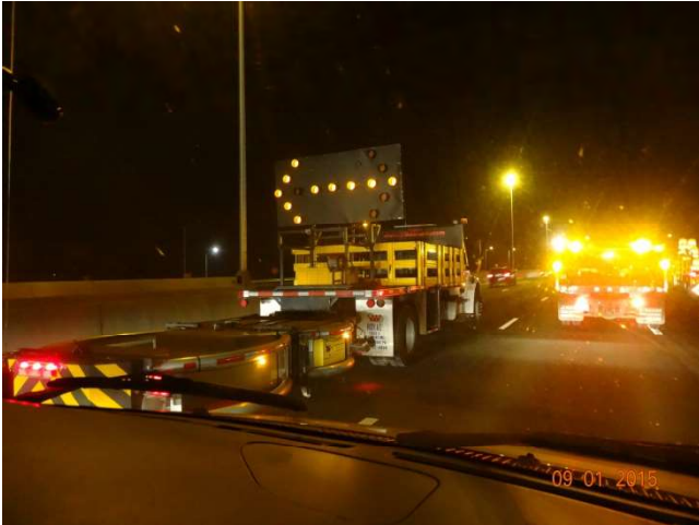
I-95 SB: A truck-mounted impact attenuator with a flashing arrow signaling to merge left.
