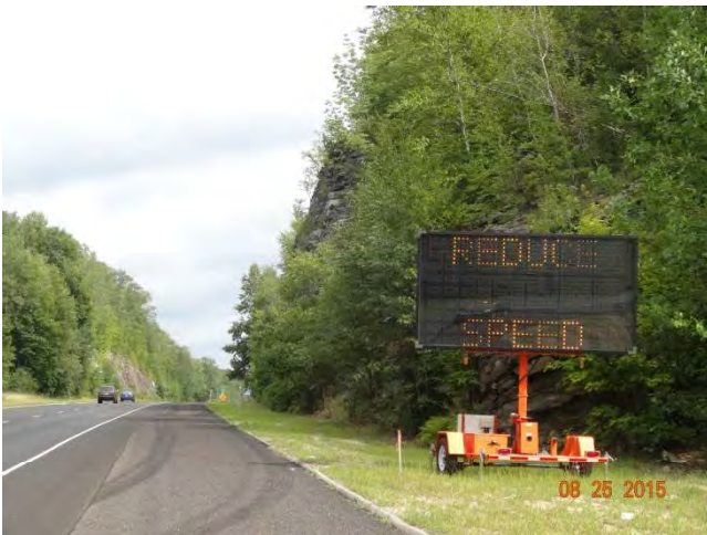
Route 11 NB: A CMS just before Exit 5 stating REDUCE SPEED on its first frame.
