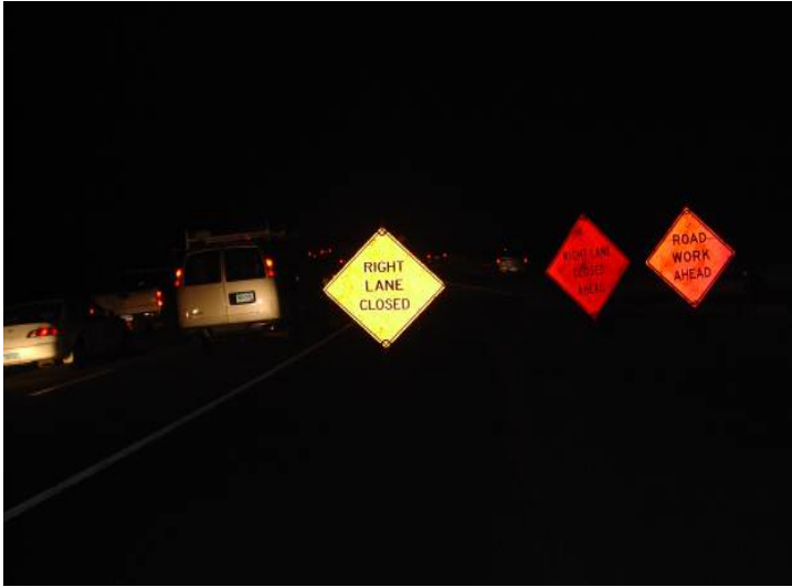
Type III Reflective sheeting (left) Versus Bright Fluorescent Sheeting
