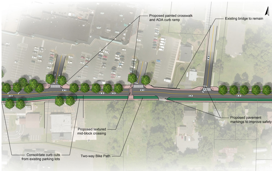
Warehouse Point Connectivity Plan. A portion of a connectivity plan in Warehouse Point, connecting key gateways in the community with the future relocated station in Windsor Locks.
