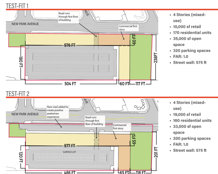
West Hartford Test Fits. Example test fits prepared for a site in the West Hartford station area.
