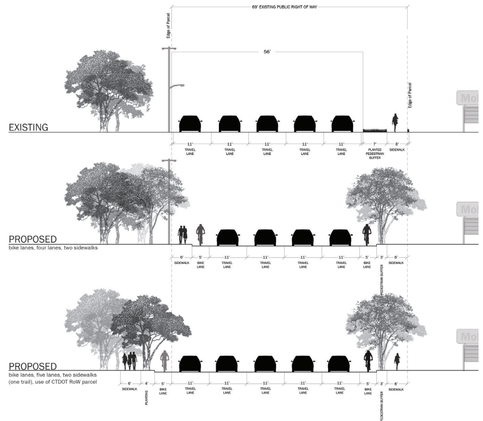
Figure 141: Fenn Road design cross-sections concepts
