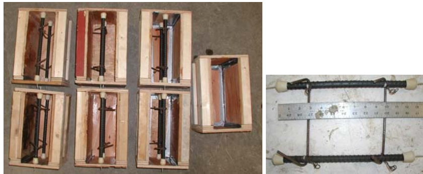
Figure 6.11: Test Slab Construction (One Set for Each Placement)
