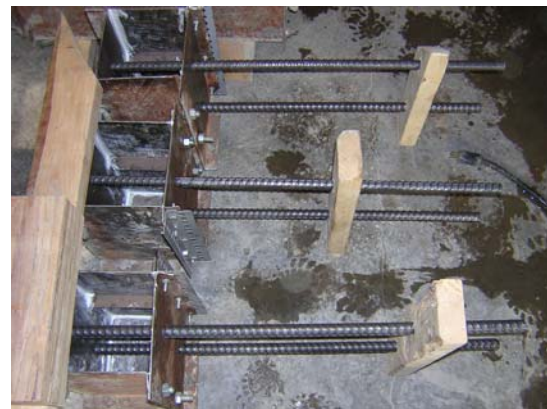
Figure 4.6: Mold for Horizontal Bars (Left to Right - ASTM Schematic/As-Used)
