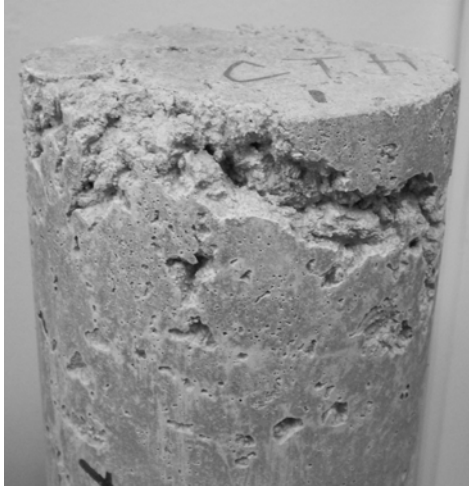
Figure 5.1: Hardened Concrete Defect Related to Hot Weather (Specimen CT687H)
