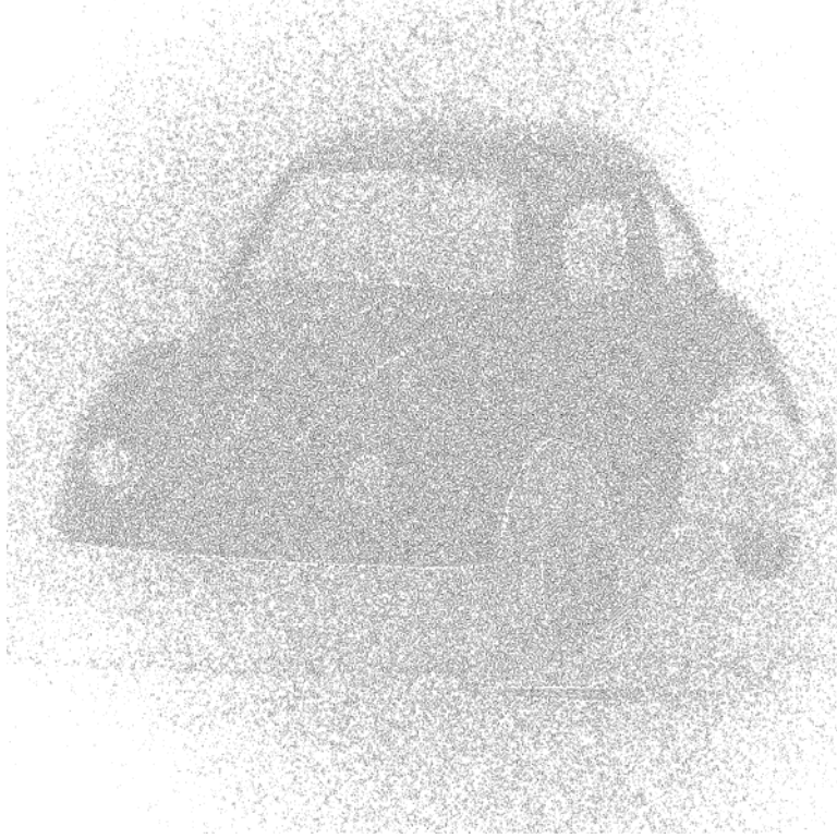
Figure 5. Edges detected in the image shown in Fig. 2(a) using the Laplacian of Gaussian – Ratio of Averages method.
