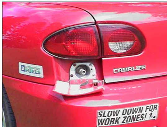
Photos 6 and 7 - Views of CNG Fuel Port Connection Located Beneath Driver's Side Tail Light
