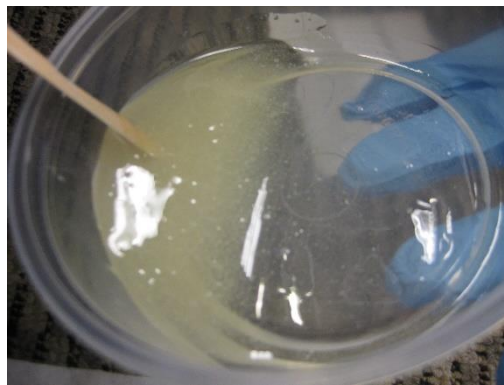
Figure 9.2 Consistency of epoxy resin and hardener mix.
