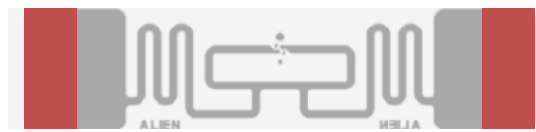
Figure 5.7 New adhesive area for sensor assembly and mounting.
