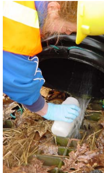
Sampling from a pipe discharge
