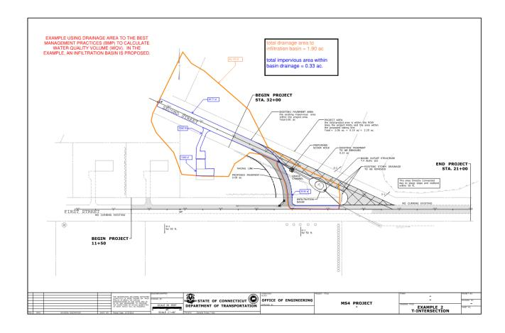
For this example, the infiltration basin is located in the excess property created by the roadway realignment. The bottom of the infiltration basin is 2 feet below the inlet elevation of the outlet structure so it will provide a two foot depth for water quality purposes. A Type 2 preformed scour hole (18' long) will be installed at the drainage system outlet to serve as pretreatment.
