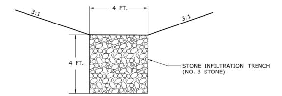
Determining the volume of the void space of the infiltration trench (assuming the stone porosity of 0.3.):
