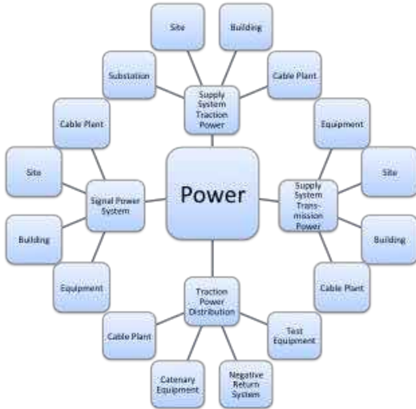
Figure 7. Asset Hierarchy – Fixed Guideway – Rail – Power
