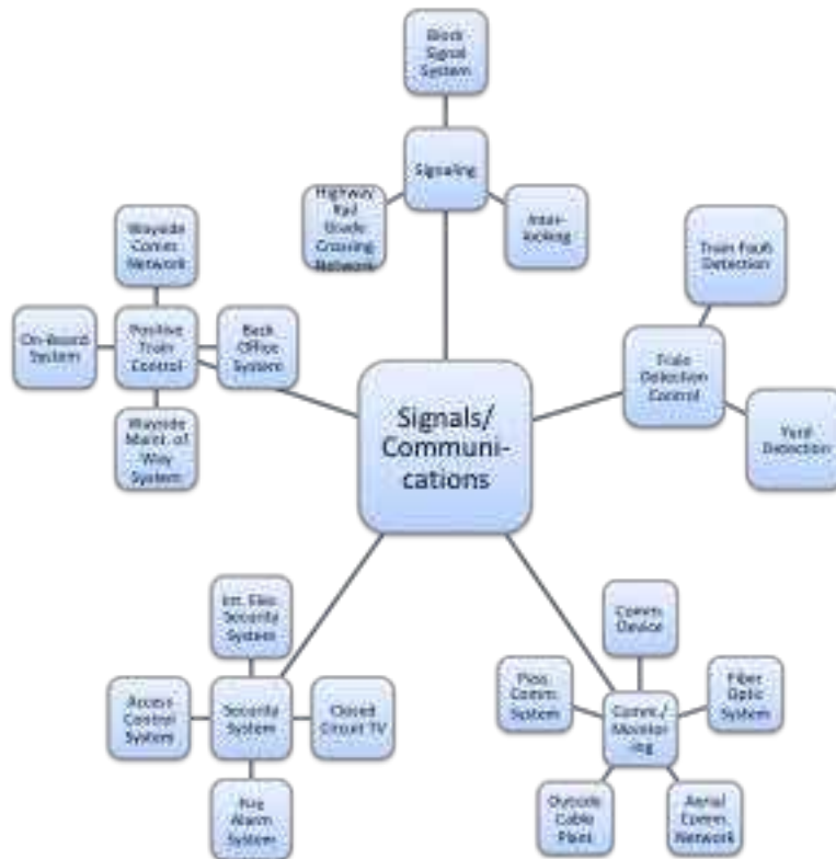
Figure 9. Asset Hierarchy – Fixed Guideway – Rail – Signal/Communications
