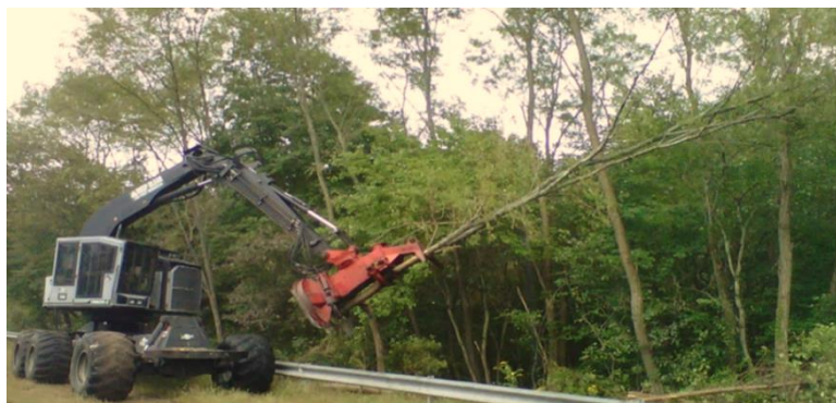
Route 9 Deep River - Feller buncher placing tree butts on an angle away from the direction of travel
