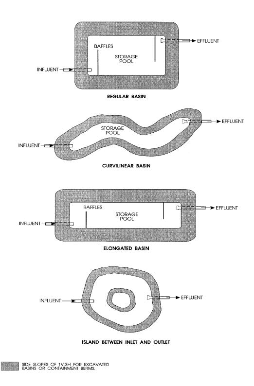
Figure 10-28 Methods Of Increasing The Length-to-Width Ratio (after Schueler, 1987)
