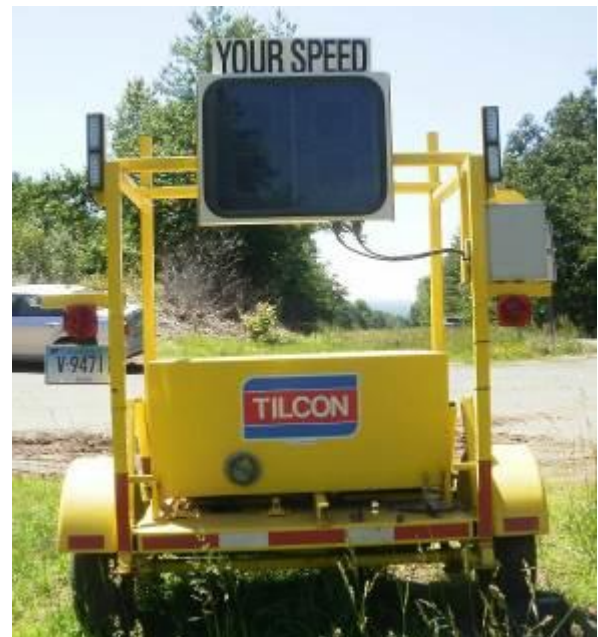
Contractor took initiative to install speed radar that operates during nighttime operations
