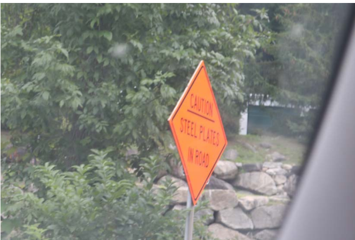
Right at the bridge is a sign stating CAUTION: STEEL PLATES IN ROAD . This sign may be better placed more in advance of the bridge.
