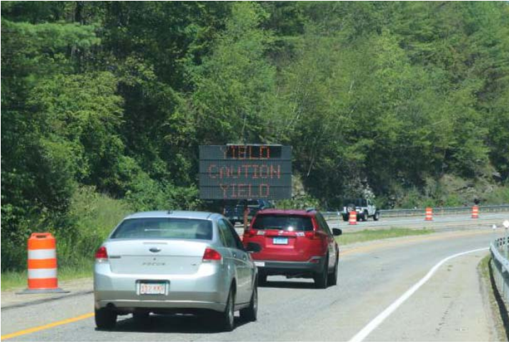
I-395 NB, Exit 94 On-Ramp: The second frame states “YIELD CAUTION YIELD”.
