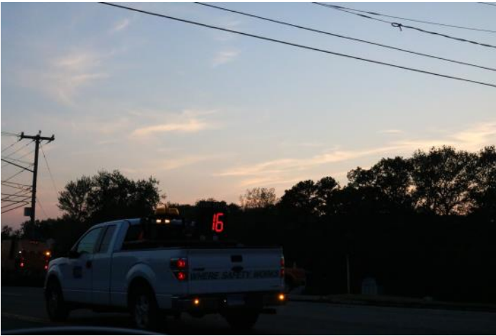
The Contractor has a truck-mounted speed trailer which is placed within the pattern.
