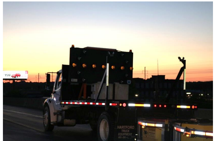
I-95 SB: A TMA used to close on ramps during the RRB had a flashing straight bar to indicate lane closed.
