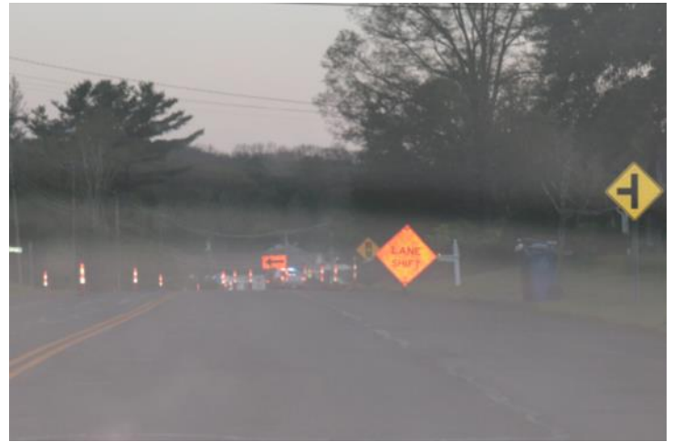
Route 6, Chaplin: This pattern uses the LANE SHIFT sign.
