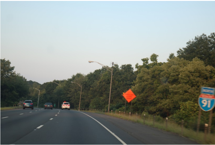
I-91 SB: A post-mounted SHOULDER CLOSED AHEAD sign.
