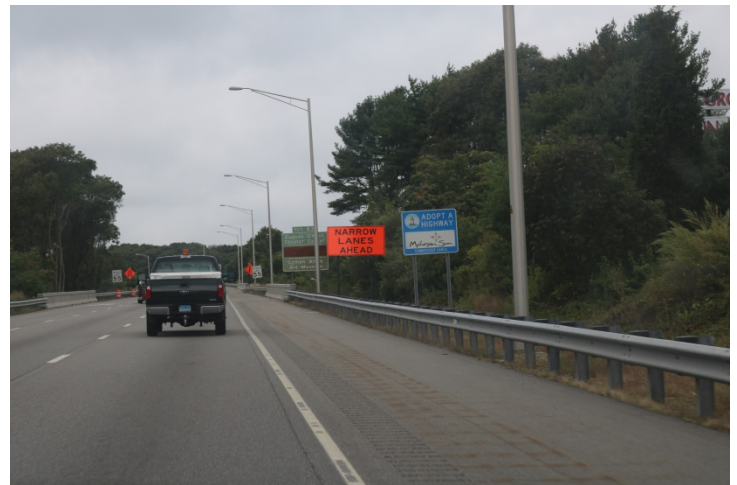
I-95 SB: A construction sign with a non-standard size states "NARROW LANES AHEAD".
