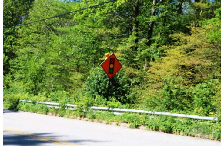
Tracy Road: A temporary signal ahead sign posted. Since it is a diamond-shaped post-mounted sign it needs a barricade warning light attached which it has.
