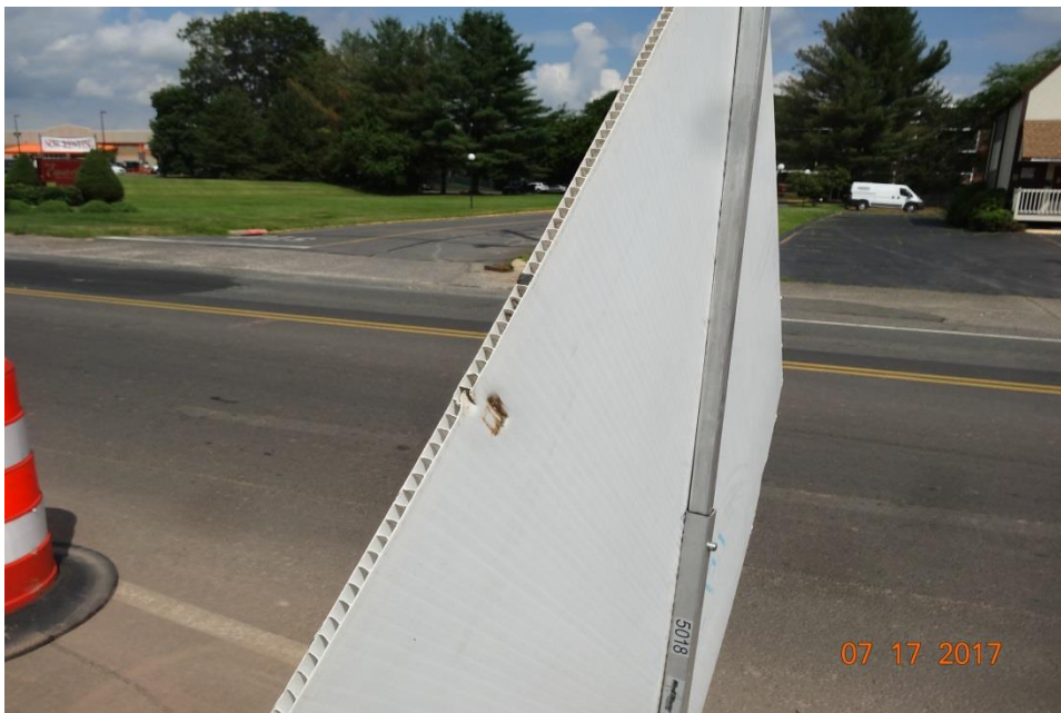
Photo 9: Corrugated plastic signs (waffle board substrate).
