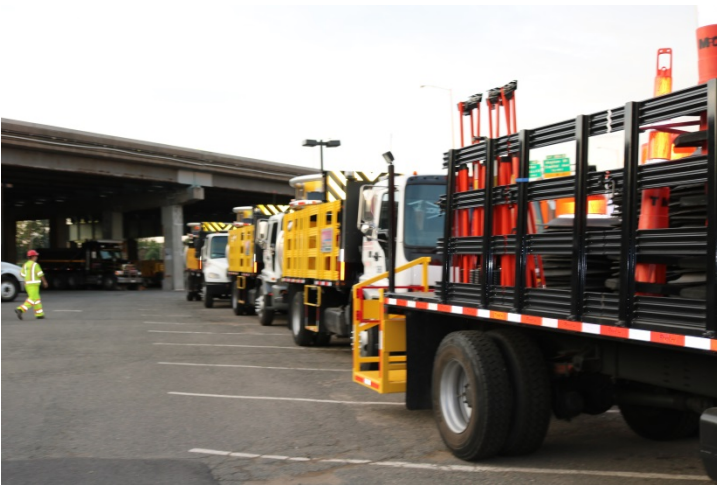
There are three out of the four crash trucks ready to proceed out on the roadway with the sign pattern truck.
