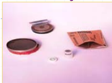
Passive device: charcoal test kits
