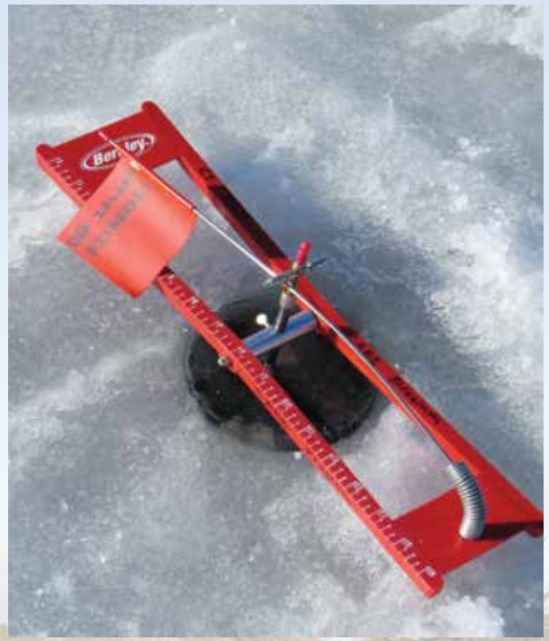
A tip-up is a device commonly used while ice fishing. The spring loaded flag “pops up” when a fish takes the bait.
