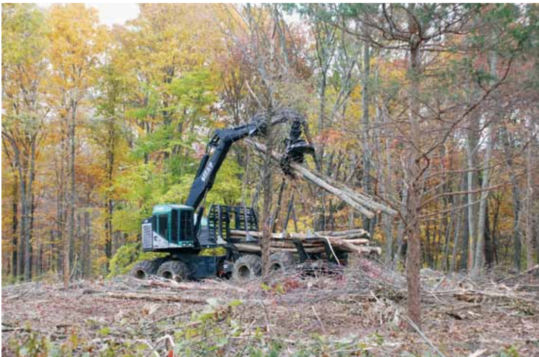
This specialized, low impact forestry equipment, called a "forwarder," was used to move trees that were cut on the Chase property to a log landing near the road.
