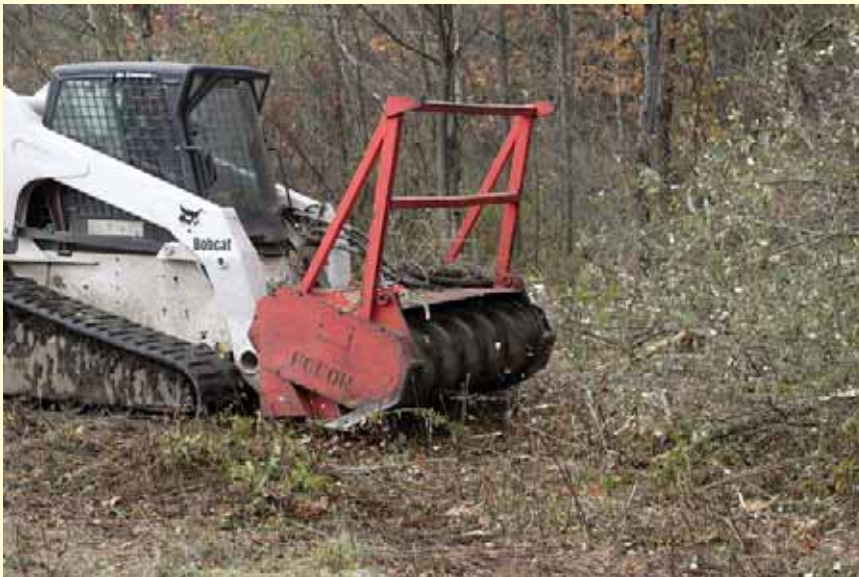
A brush hog was used at Mad River Flood Control Area in Winchester to maintain early successional stage habitat.
