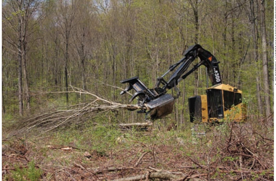
A feller buncher is used to clear an area at Bishop Swamp Wildlife Management Area in Andover for the regeneration of aspen.
