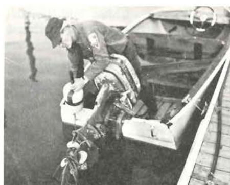
Toward the end of the day we meet C. O. George Hayden at an unpleasant task—checking a recently-submerged boat whose prop had fouled in a lobster pot line and apparently caused two fatalities.
