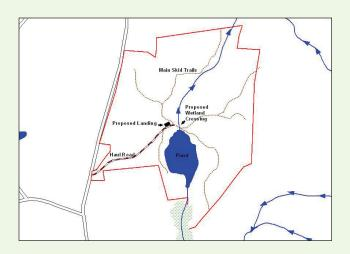
To minimize potential problems, the **operational plan** must consider soils and topography of the area. Planned erosion and sedimentation controls must be both effective and practical. A variety of tools can help in evaluating the site and developing a plan for harvesting activities before entering the site. Useful tools may include: topographic maps, aerial photos, U.S.D.A. soil maps, property maps, tax maps or municipal wetland maps.
