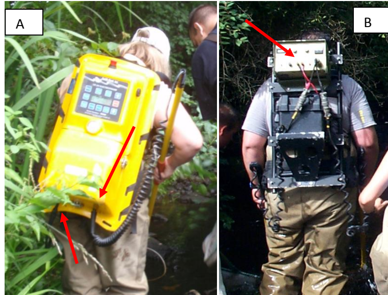
Figure 4.6a-b. Two backpack electrofishing models- Smith-Root (A) and Coffelt (B). Anode and cathode connections are located on the bottom of Smith-Root models (A, left) and on the top of the Coffelt models (B, right).
