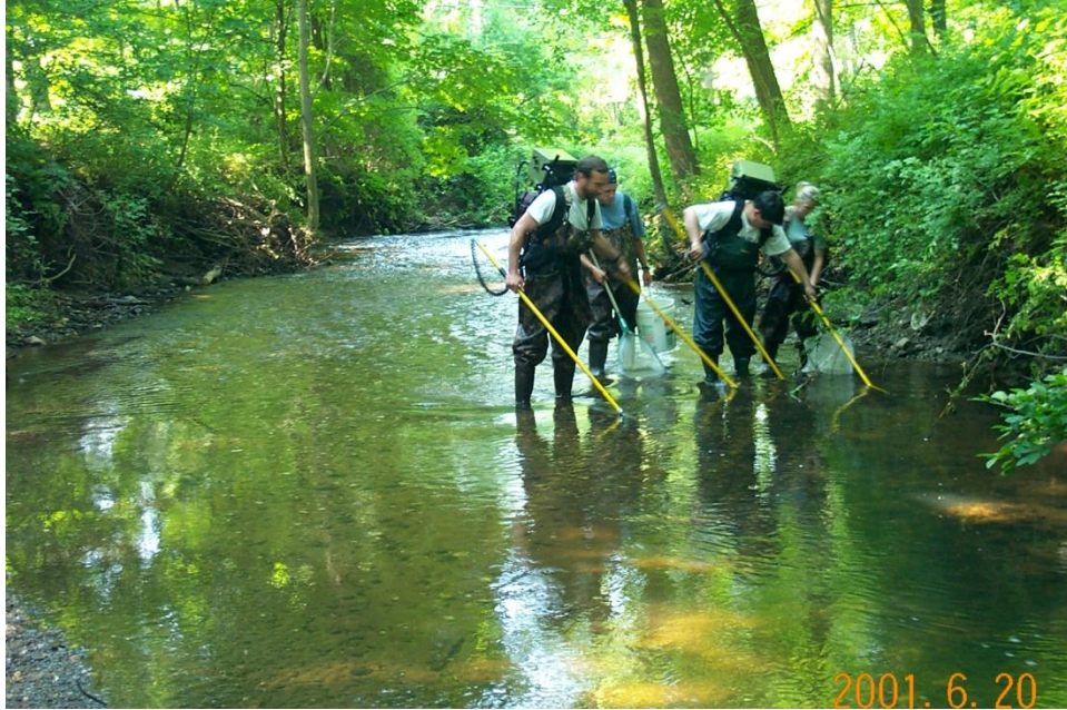
Figure 4.4. Crew configuration will vary depending on the number of crew members available and the width and depth of the stream to be sampled. Shown above is a four-person crew with two backpack units and two netters. In this case, one netter also maintains the collection bucket.
