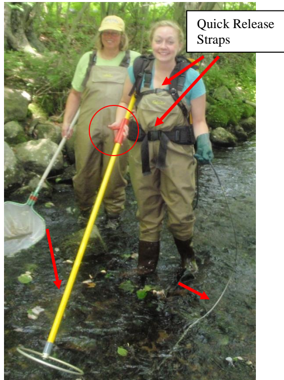
Figure 4.5. A Smith-Root backpack Electrofisher. The black rat tail is visible in the operator's left hand and the anode (pole with ring) in her right hand. Note the red on/off switch located on the anode pole handle. (Note that the switch is in the open/off position and the anode has been removed from the water ensuring there is no chance that a crew member will be shocked. During electrofishing the rat tail is placed behind the operator.)
