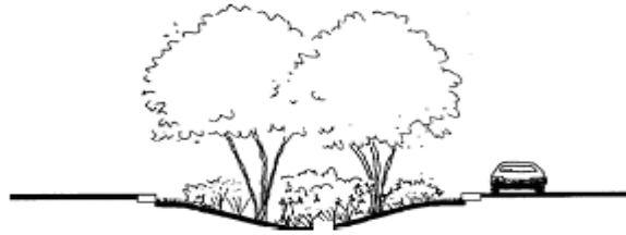
Figure 6.4.10 – Cul-de-sac infiltration island accepts stormwater from surrounding pavement. Note flat curb. Source: Connecticut, 2004.
