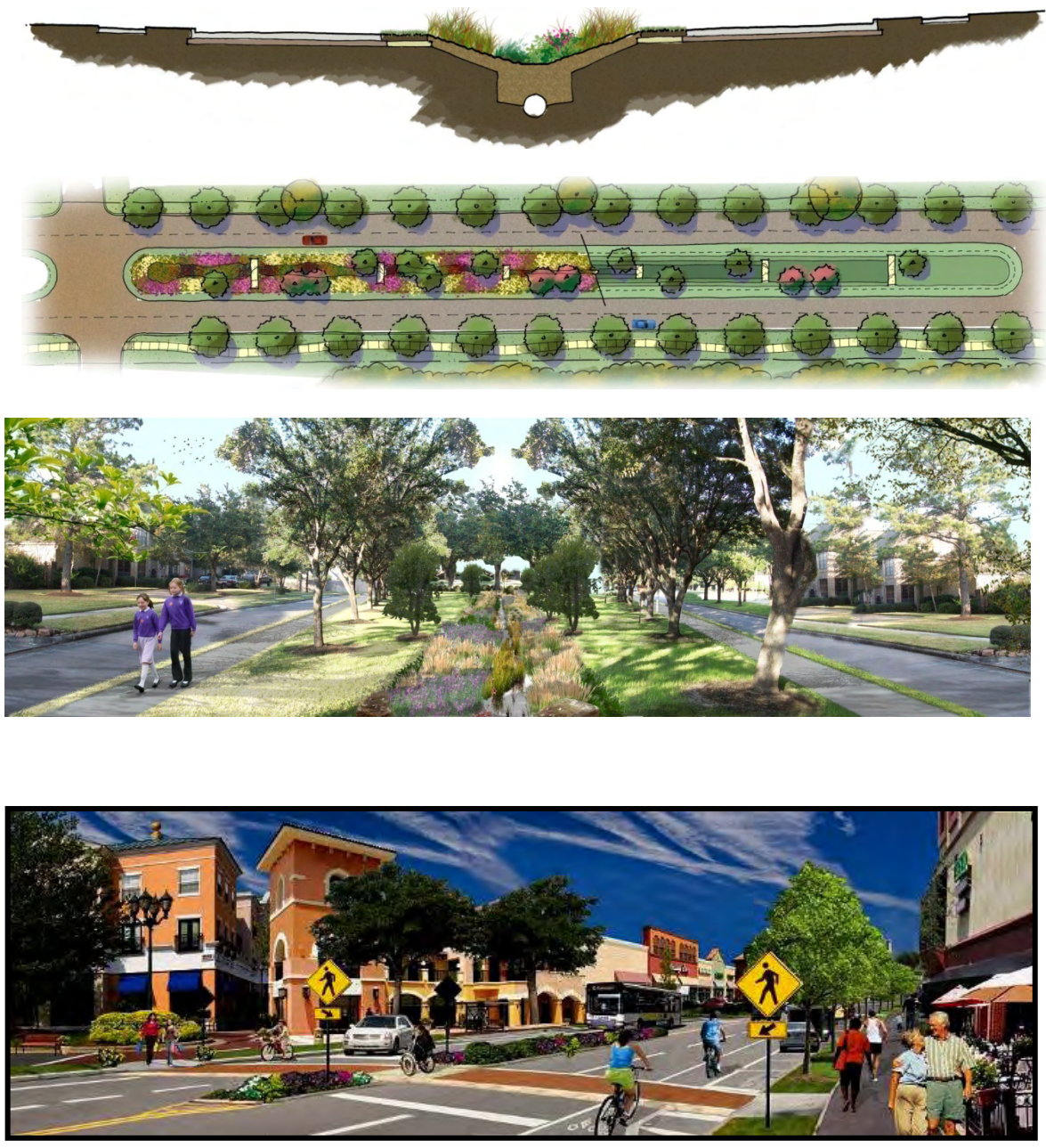
Figure 6.3.8 – Examples of center median infiltration/filtration systems.
