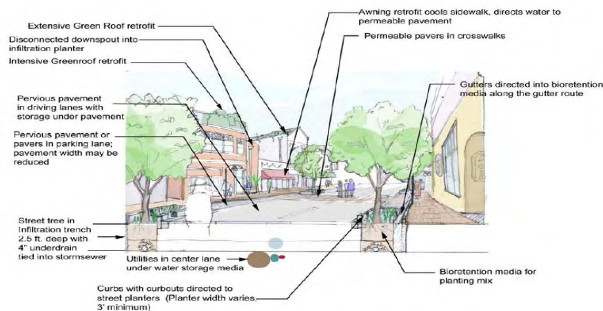
Decentralized Stormwater Controls in Urban Retrofit Streetscape
