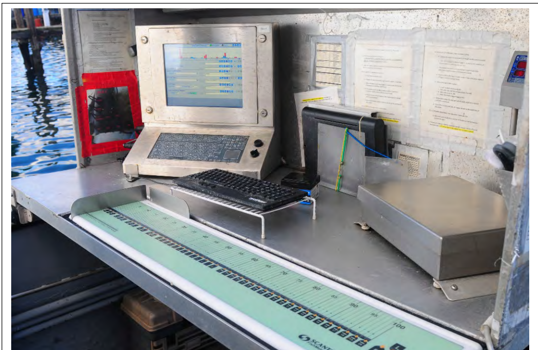
An electronic measuring station on the NEAMAP trawl survey.
