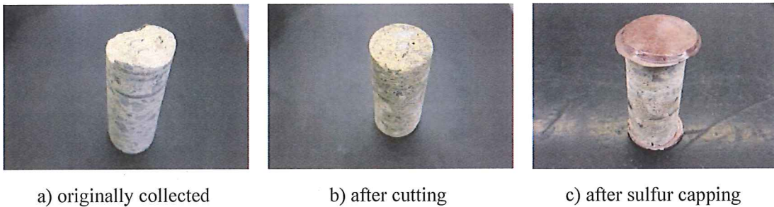
Fig. 4.2 Specimen preparation procedure
