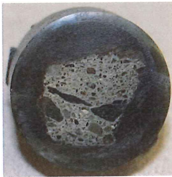
a) samples impregnated with low viscosity resin
