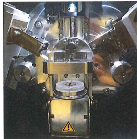
f) sample mounted for XRD test
