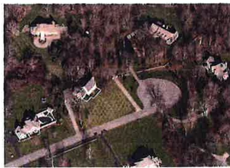
Typical offset cul-de-sac (60ft. radius)
