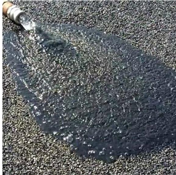
Pervious pavement can be applied as sidewalks, streetscaping areas, parking lanes, gutter strips or entire roadway surfaces. Such treatments are effective where landscape-based improvements aren't feasible or desired.
