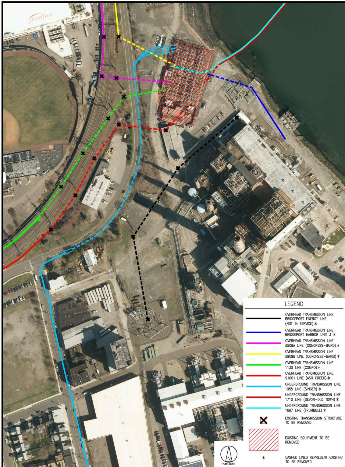
**Figure ES-3: Existing Conditions: Proposed Site for Rebuilt Pequonnock Substation**
