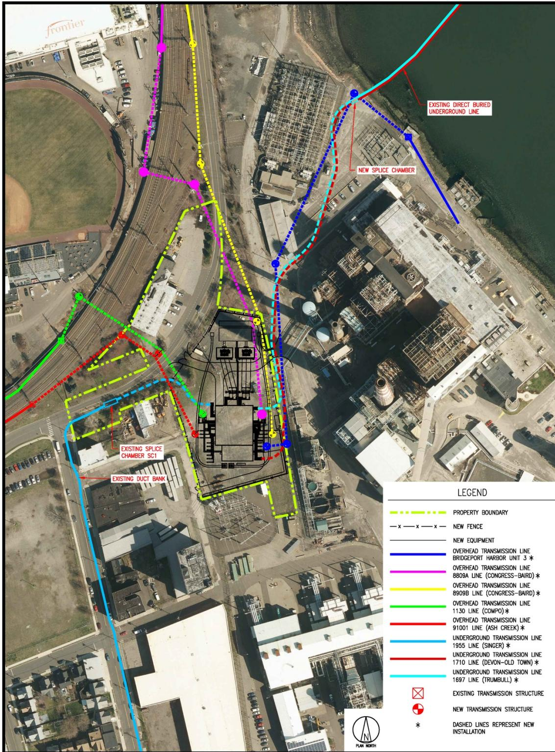
Figure 1-6: Existing Pequonnock Substation and 115-kV Line Connections to be Decommissioned
