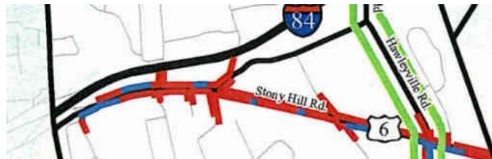
ROUTE 6 IN BETHEL SHOWING EXISTING SIDEWALKS IN BLUE AND NEEDED ADDITIONS IN RED, AS EXCERPTED FROM THE 2007 BETHEL PLAN OF CONSERVATION AND DEVELOPMENT
