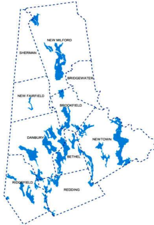
Major stratified drift (sand and gravel) aquifers in the Housatonic Region are found in the lowlands of river valleys
