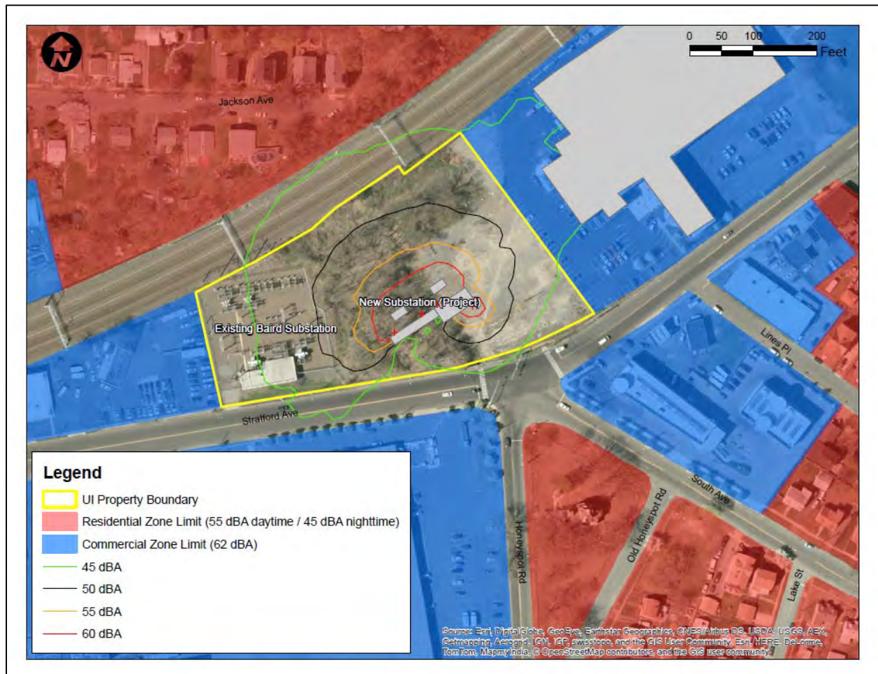
Figure 4-1 Project A-weighted sound pressure levels, normal operation consistent with Summer months.
