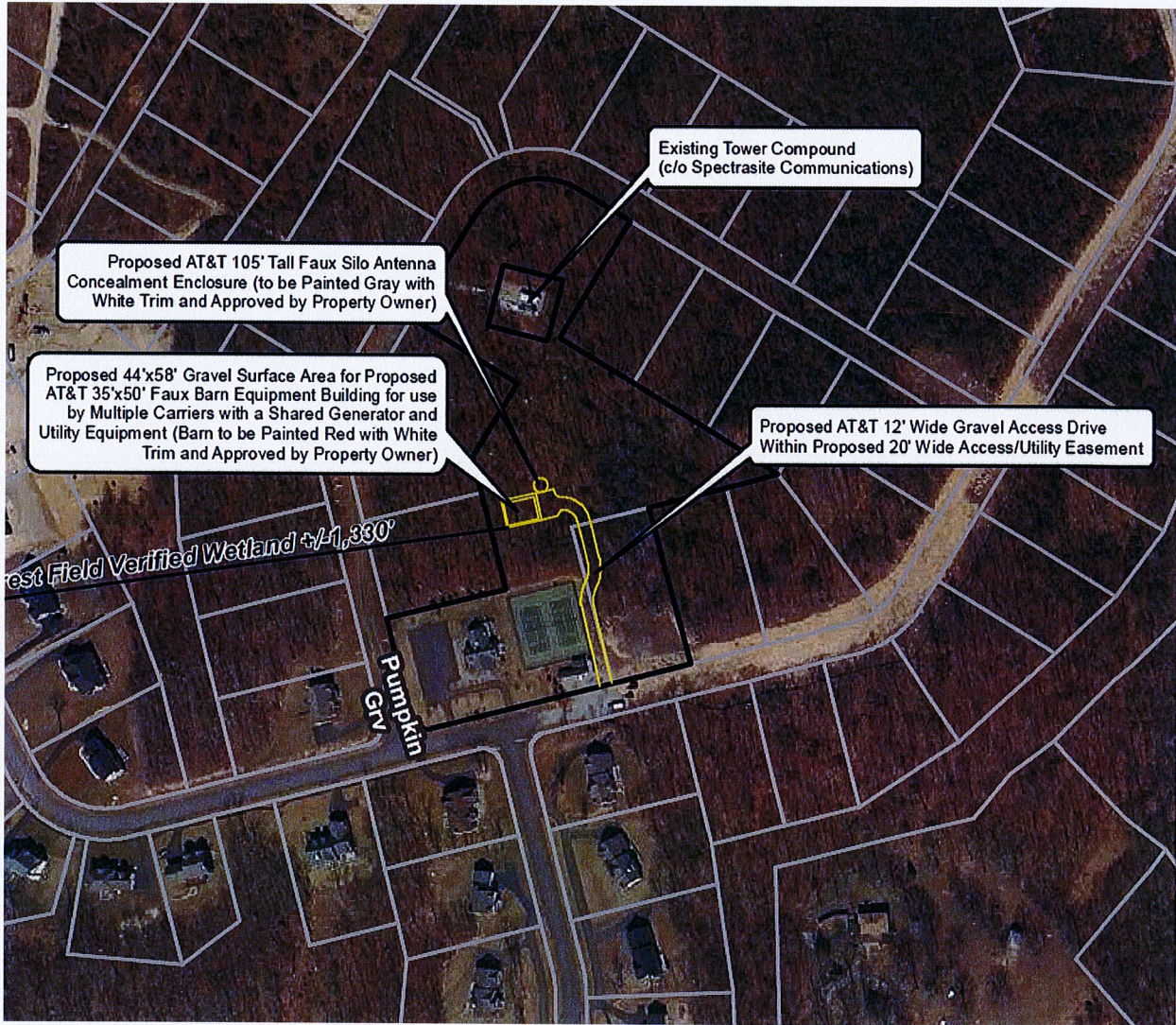
Figure 5 – Aerial Photograph Showing Existing Tower at 2 Scott Road and the proposed 2 Arbor Crossing facility.
