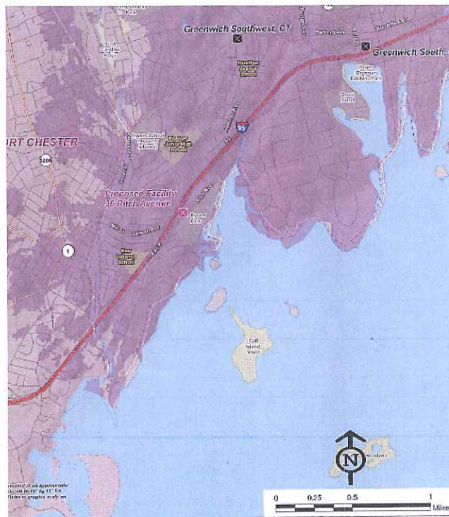
Figure 5: Cellco existing and proposed PCS coverage at -85 dBm. (Cellco 1, Tab 6; Cellco 4, R. 4)
