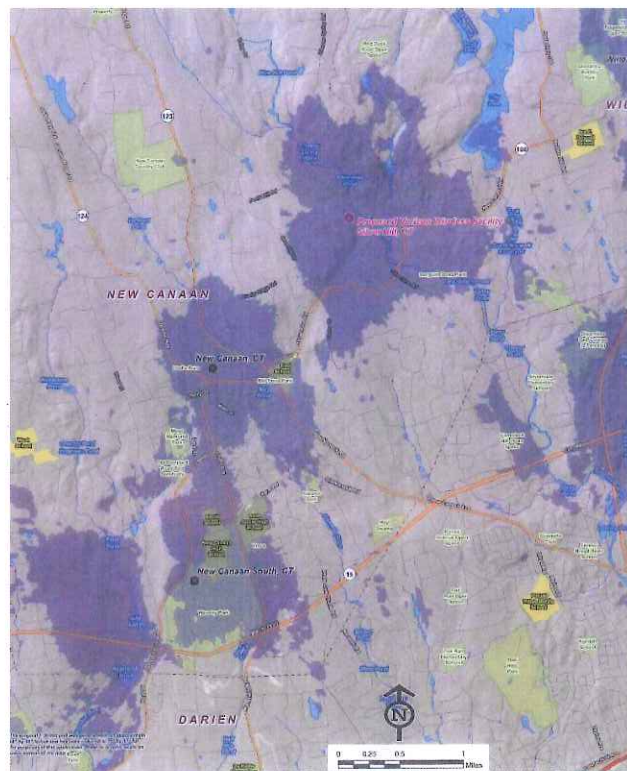
Figure 10. Existing Cellco PCS coverage and coverage from the proposed site at 97 ft. agl. (Cellco 1, Tab 2)
