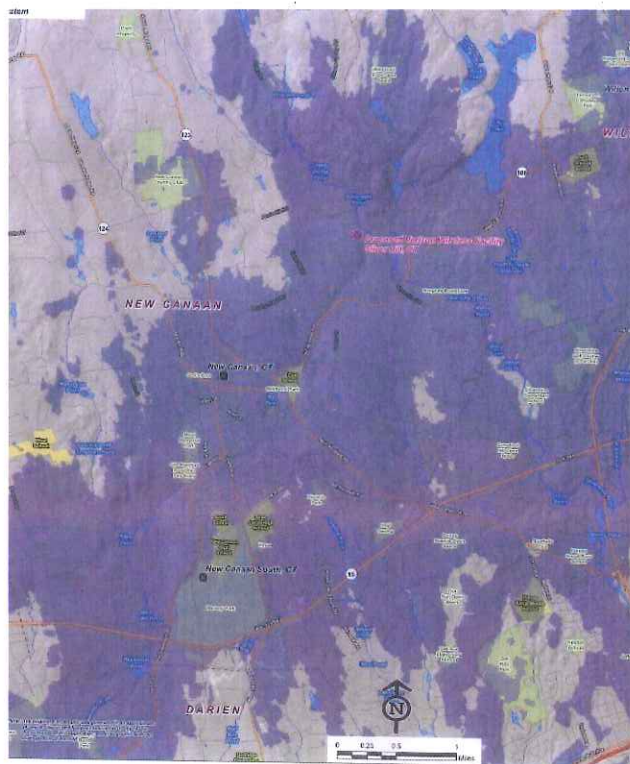
Figure 8. Existing Cellco LTE coverage and coverage from the proposed site at 97 feet agl. (Cellco 2, Tab 1)
