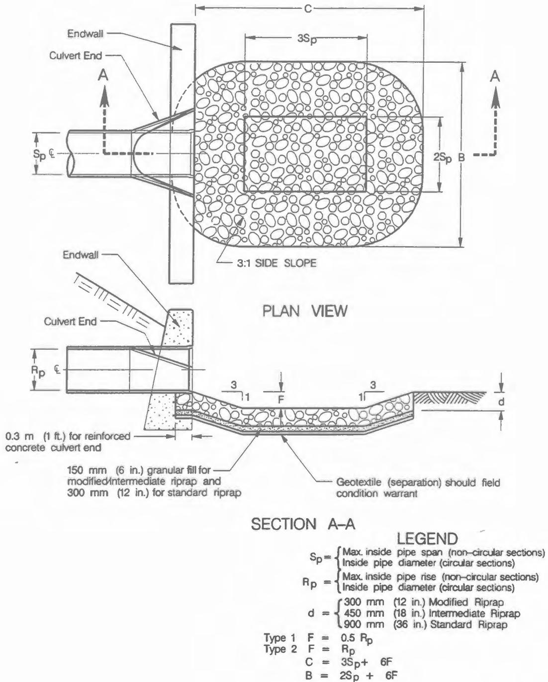
Figure 8-11 Preformed Scour Hole Type 1 and Type 2
