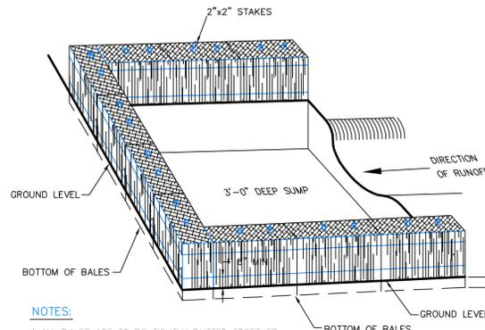
**WATER BAR - TEMPORARY DIVERSION DITCH WITH HAYBALE TRAP**
