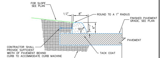
**BITUMINOUS CONCRETE CURB DETAIL**
