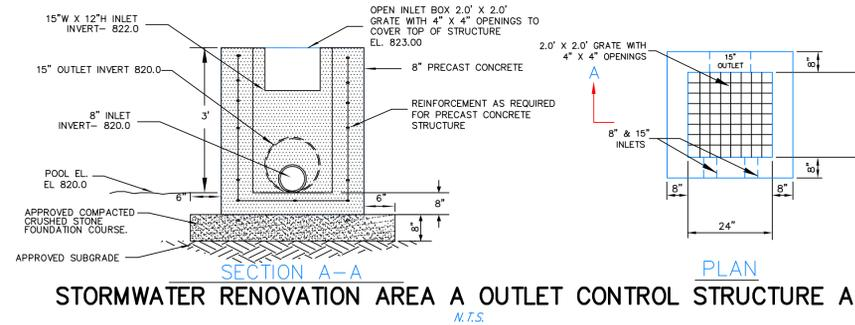
STORMWATER RENOVATION AREA A OUTLET CONTROL STRUCTURE A
