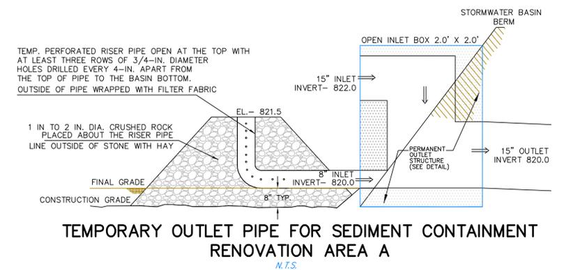
TEMPORARY OUTLET PIPE FOR SEDIMENT CONTAINMENT RENOVATION AREA A
