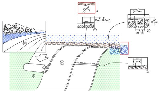
1. PREPARE SOIL BEFORE INSTALLING BLANKETS, INCLUDING ANY NECESSARY APPLICATION OF LIME, FERTILIZER, AND SEED. NOTE: WHEN USING CELL-O-SEED DO NOT SEED PREPARED AREA. CELL-O-SEED MUST BE INSTALLED WITH PAPER SIDE DOWN.
