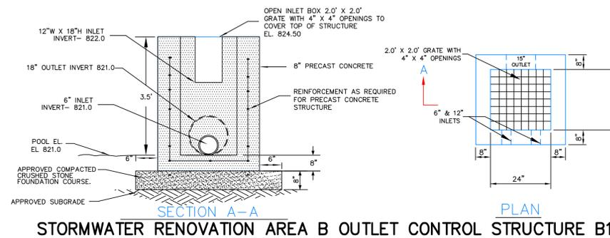
STORMWATER RENOVATION AREA B OUTLET CONTROL STRUCTURE B1
