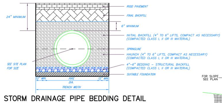
**STORM DRAINAGE PIPE BEDDING DETAIL**
