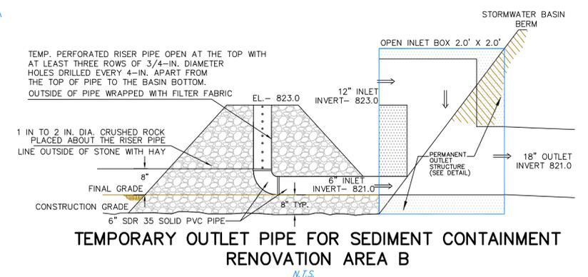
TEMPORARY OUTLET PIPE FOR SEDIMENT CONTAINMENT RENOVATION AREA B
