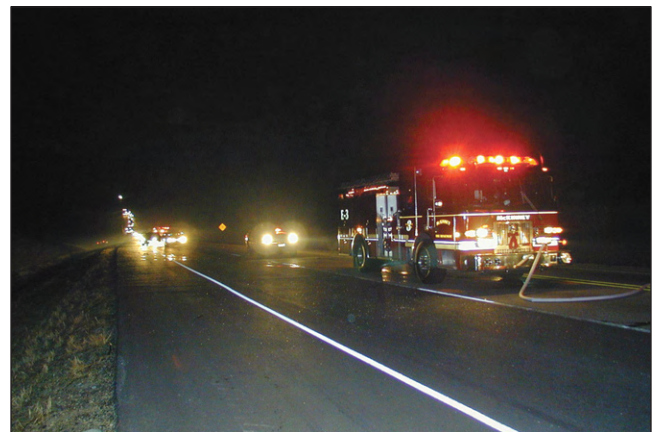
Figure 6.7—Minimize lighting at night so as to avoid blinding approaching drivers. Courtesy of Ron Moore, McKinney, TX FD.
