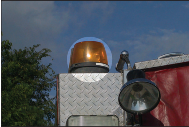
Figure 4.8a—These amber lights are mounted on the rear of the apparatus.
