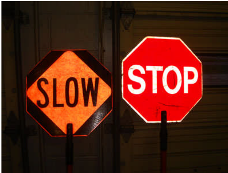
Photo 4. Traffic control devices used by Unit 1911. (NIOSH photo)
