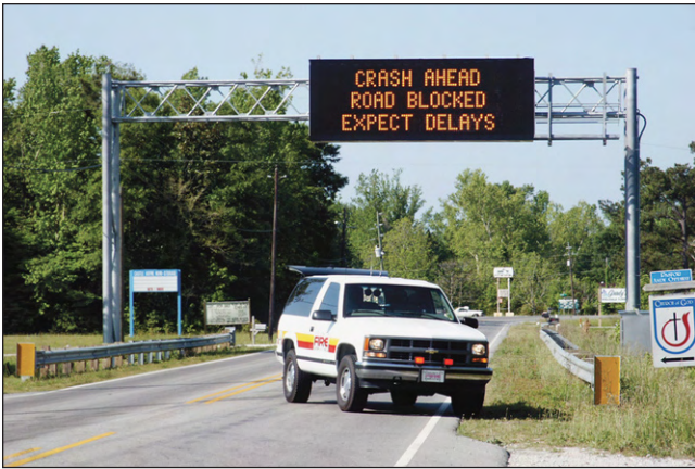
Figure 3.3—Variable message signs provide advanced warning to approaching motorists. Note that the DOT would prefer the use of the term “Crash Ahead” rather than “Accident Ahead.”
