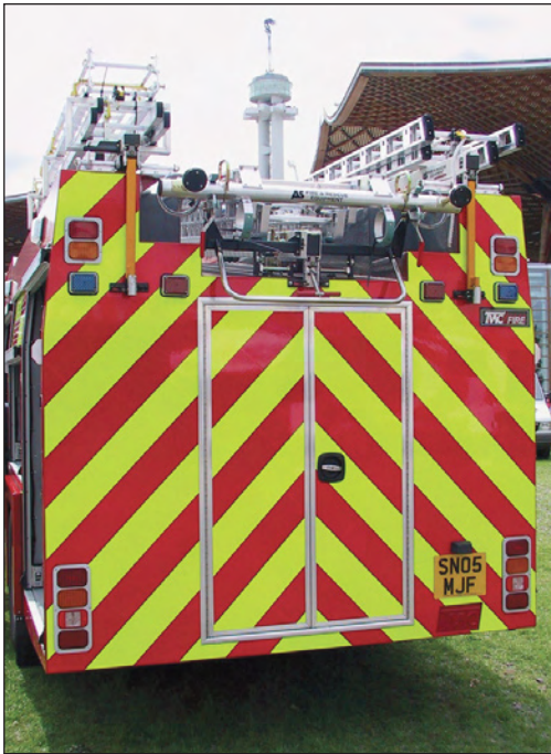
Figure 3.24—European fire apparatus have used reflective marking on the rear of their apparatus for many years.
