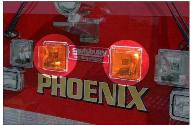
Figure 4.8b—Some departments place amber flashers on all sides of the apparatus.
