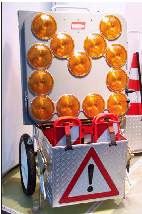
Figure 3.28—This traffic control cart includes a battery-operated arrow board.
