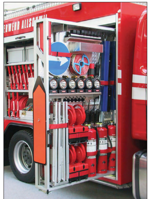
Figure 3.26—German fire apparatus commonly have whole compartments dedicated to carrying traffic safety equipment.
