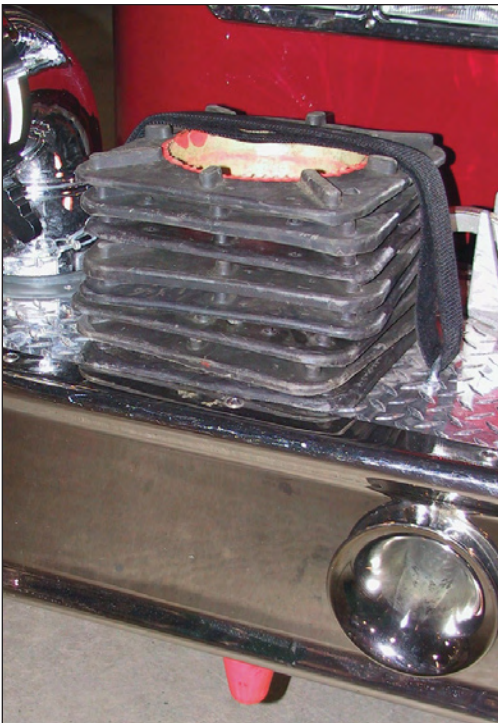
Figure 3.8—This department designed a place to store traffic cones in the extended front bumper of the apparatus.
