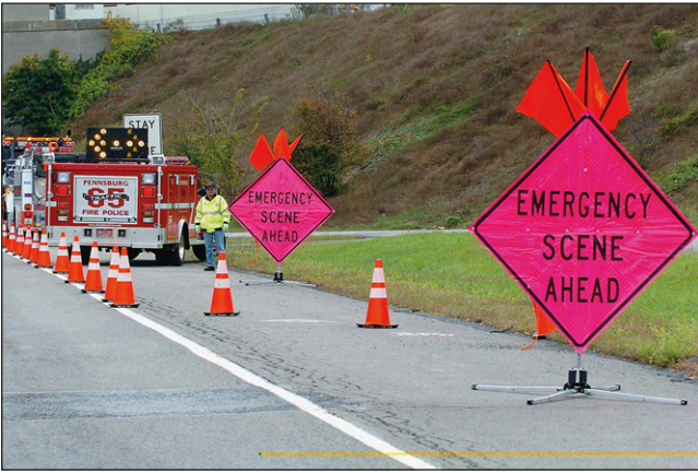
Figure 3.6—NFPA 1500 requires the use of pink “Emergency Scene Ahead” signs on roadway incidents.
