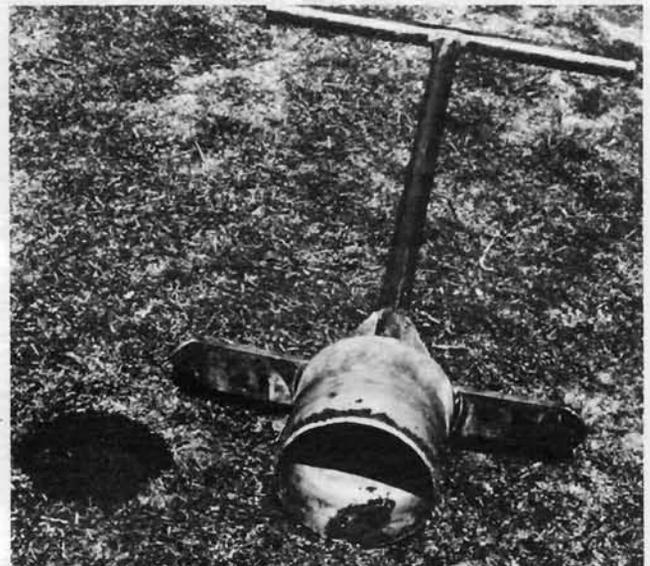
Fig. 2. Core sampler used in examining soil for Japanese beetle grubs; diam. = 6.4 inches.
