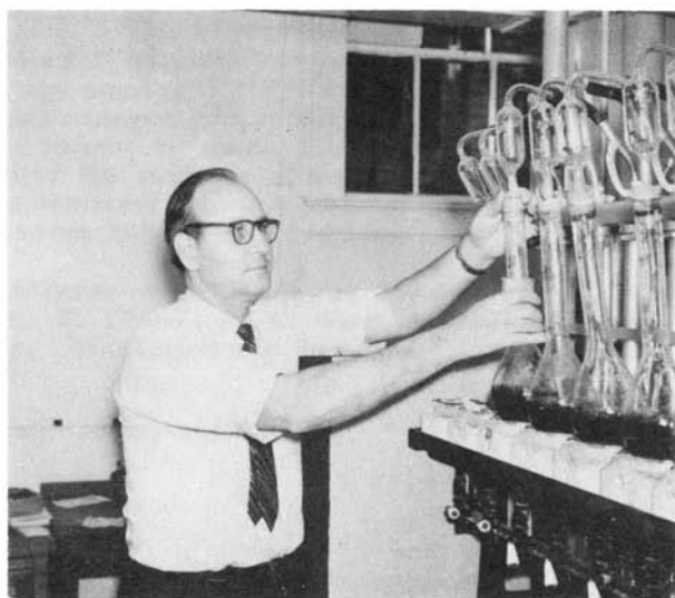
William Glowa makes nitrogen determination.
