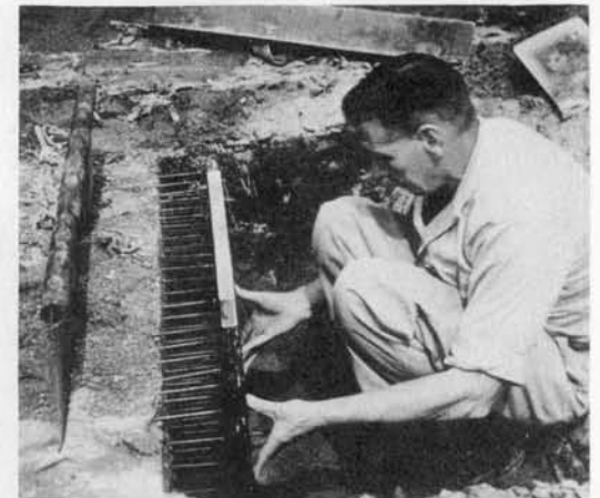
FIGURE 6. The pin-board is driven into the soil profile so that the board touches the face of the trench. The bottom plate, shown in background, is driven into place before the monolith is cut free.
