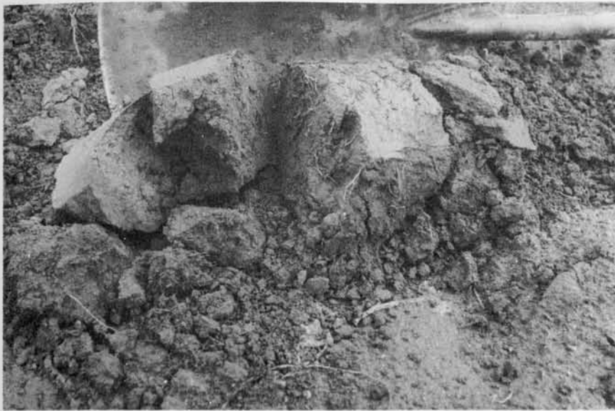
FIGURE 4a. After-harvest spade test of Merrimac sandy loam in a Havana Seed field shows that 18-inch slice breaks into two main sections: furrow slice or plow layer at the right, compaction layer on the left. The massive-structured plow layer is capped by a crumbly to subangular blocky cultivated zone. No roots penetrated the compaction layer.
