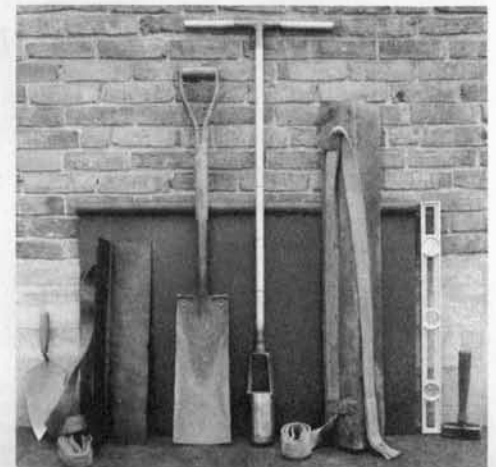
FIGURE 7. Root-sampling tools and equipment: when the short bottom plate is used the steel sheet is turned and an auger hole made for the pipe-rim.
