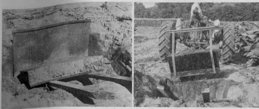
FIGURES 8 and 9. Soil monolith with root sample resting on the pin-board and bottom-plate, cut free by steel sheet, ready to be slid from the pit. (Right) A monolith, inner face cut with long spade, lifted and transported by the hydraulic lift on tractor.
