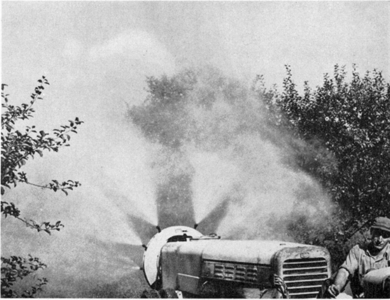
Figure 19—The Hurst hang-on equipped with nozzles shown in Figure 7. This outfit is equipped with fixed directional vanes (not shown).
