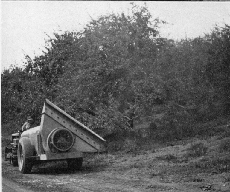
Figure 15—The Hardie "Orchard Mist" provided with T-jets and movable vanes in slot for directing the spray. This machine is designed for concentrates.
