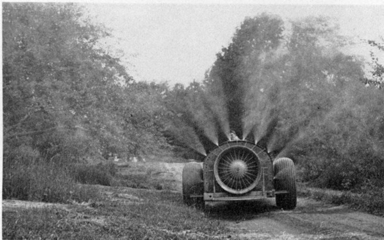
Figure 14—The Hardie King, designed for concentrates and operating from both sides. Note large size tires for ease in operation on soft ground.
