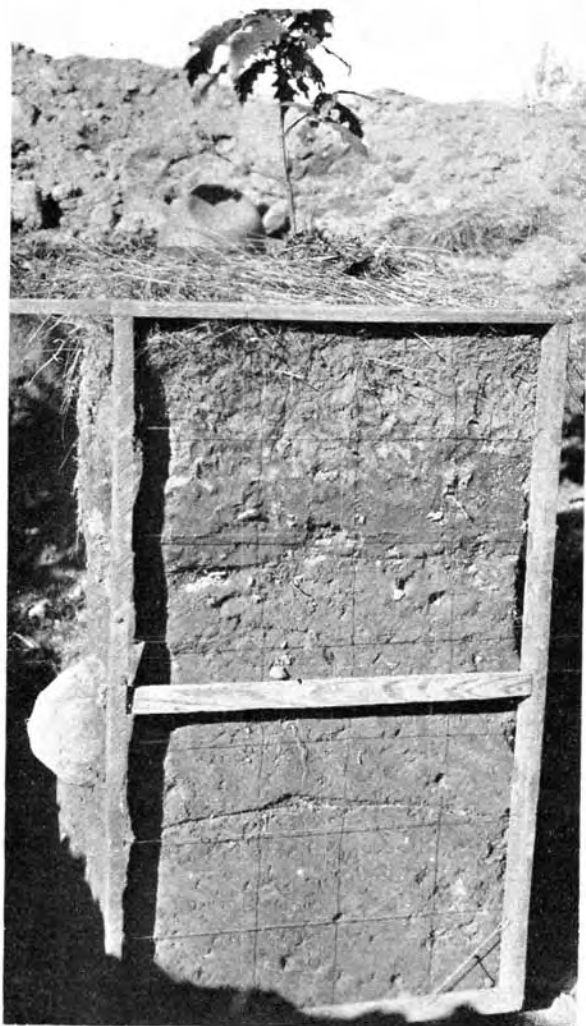
Figure 7. View of the frame used for field mapping. The frame is fitted against the 2x2 foot block of soil. Note cross-wires, 0.5 foot apart, which were used as reference lines. Exposure of typical profile in Charlton fine sandy loam, Bantam Lake, Bantam, Connecticut.
