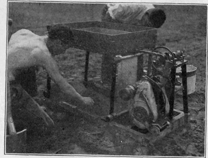
FIGURE 7. Soil sifting apparatus used for determining wireworm population in treated and untreated areas. Windsor, Connecticut, 1939
