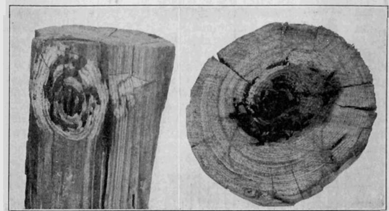
FIGURE 92. Left: section cut at an angle through the laminated part of a carpenter ant cavity in a telephone pole. Right: cross section through a treated ant cavity below the level at which the creosote was applied. The dark stain is due to creosote.
