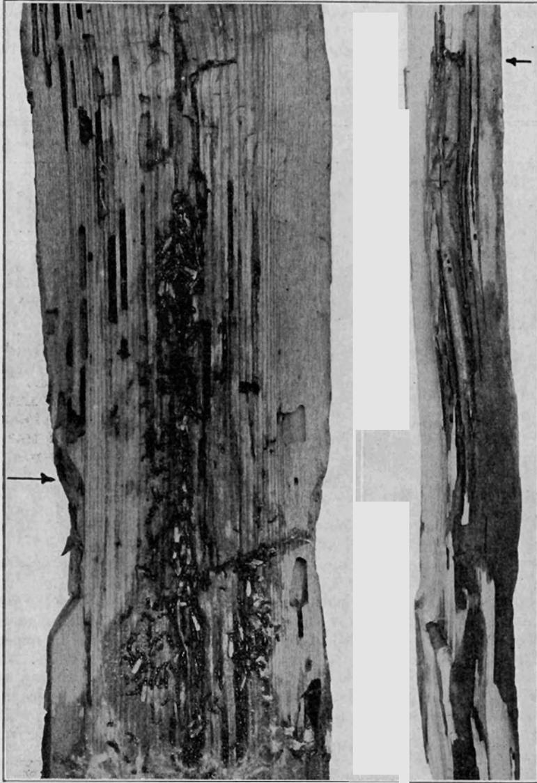
FIGURE 91. Left: carpenter ant colony in telephone pole in winter. The arrow indicates the ground level. The section is about 2 feet long. Right: longitudinal section of a treated pole. The dark stain is due to creosote injected at the level indicated by the arrow. The section is about 4 feet long.
