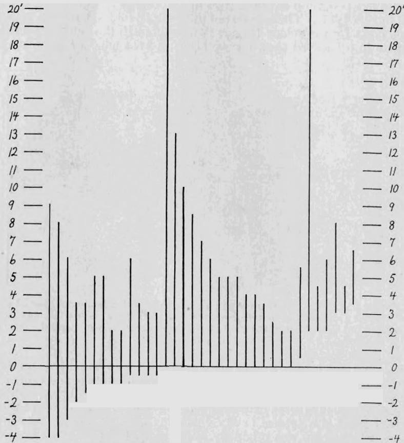
FIGURE 93. Length and position of carpenter ant cavities in 35 telephone poles. Each vertical line represents the extent of one cavity. The figures on each side represent distance in feet from the ground level (horizontal line).
